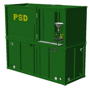
rate in to a water stream where the grains of polymer are wetted before they fall under gravity in to the mixing tank below. The flocculant feeder unit attaches to the water tank to form a standard 20 foot container sized module, complete with ISO corner castings, for transport.
